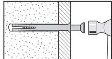
For use with walls stuck with plasterboard. The hammer fixing allows it to be fixed to the wall rather than the plasterboard. Always check the fixing is secure to the
