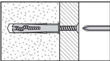
Generally aerated blocks should not be used to support heavy loads, use a specialist fitting in this case. For light loads, general purpose wall plugs can be used.
