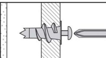
For use when attaching light loads on to plasterboard partitions.
