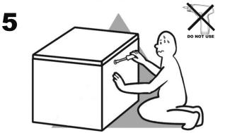
**DO NOT** fully tighten screws leave slightly loose). When the item is fully assembled tighten the screws - but do not over tighten.
