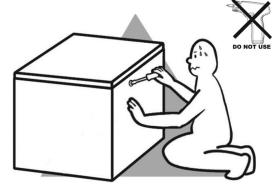
**DO NOT** fully tighten screws leave slightly loose). When the item is fully assembled tighten the screws - but do not over tighten.
