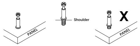
Tighten quickfit until shoulder is flush with panel. Do not overtighten or undertighten.
