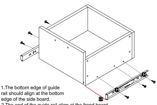
2. The end of the guide rail align at the frond board.
